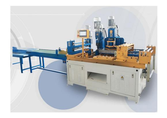
A silicon steel transformer core cutting machine uses servo motors to feed, punch, and cut electrical silicon steel coils into rectangular laminations. These laminations are used for transformers, welders, and reactors.
